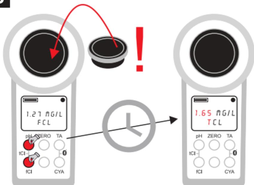
Total Chlorine is measured directly after free Chlorine without emptying the cuvette. The DPD 3 tablet is added to the sample water which already contains the DPD 1 tablet (dissolved). Combined Chlorine is calculated as
