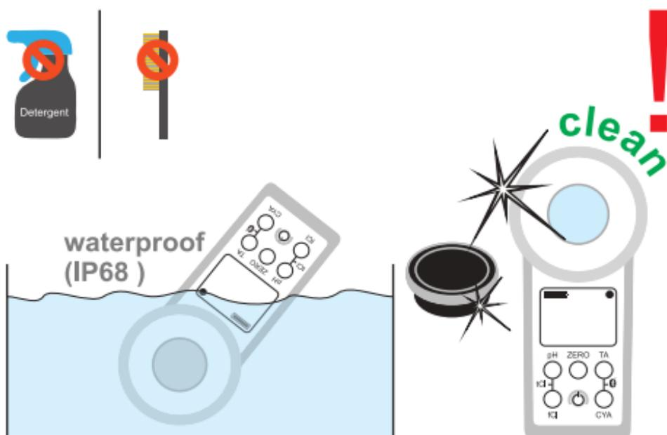
It is important to clean the device after each measurement to get rid of any reagent residues!
