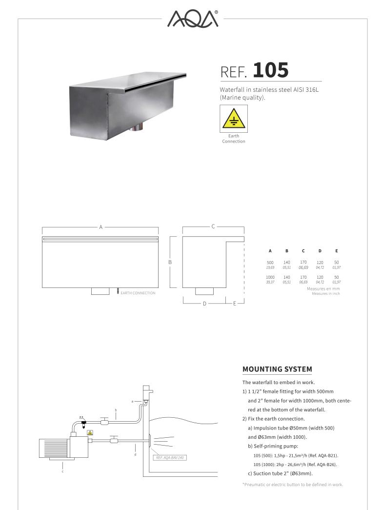
\*\*AQA recommends to install a POOL PROTECTOR to avoid corrosion of the existing stainless steel elements in the pool.
